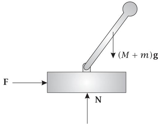
**Figure 4-2** Free Body Diagram of Block-Particle System for Question. 4-1
