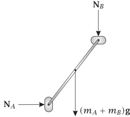
**Figure 4-5** Free Body Diagram of System for Question 4-17.
