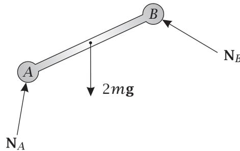
**Figure 4-7** Free Body Diagram of System for Question 4-17.
