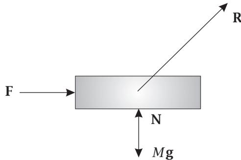
**Figure 4-1** Free Body Diagram of Block for Question. 4-1
