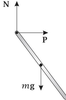
**Figure 5-19** Free Body Diagram of Rod for Question 5–11.
