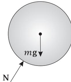
**Figure 5-8** Free Body Diagram of Cylinder During Frictionless Segment for Question 5-5.
