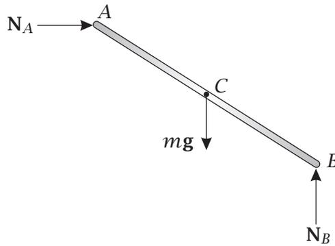
Figure 5-11 Free Body Diagram of Rod for Question 5.7.
