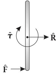
**Figure 5-7** Free Body Diagram of Rod During Application of  $\hat{\mathbf{F}}$  for Problem 5–4.
