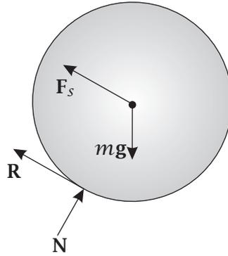
**Figure 5-16** Free Body Diagram of Cylinder for Question 5–10.
