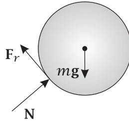
**Figure 5-15** Free Body Diagram of Rolling Sphere for Question 5–8.
