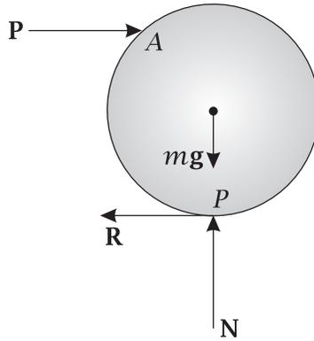
Figure 5-22 Free Body Diagram of Rod for Question 5-16.
