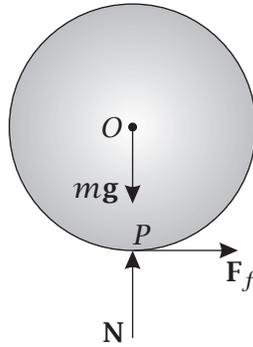
**Figure 5-1** Free Body Diagram of Disk
