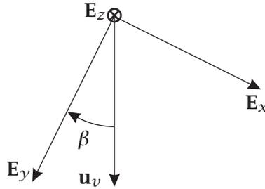
**Figure 5-10** Free Body Diagram of Cylinder During Segment with Friction for Question 5–5.
