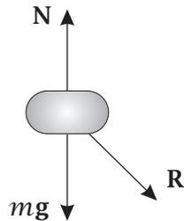
**Figure 5-3** Free Body Diagram of Collar for Question 6.2.
